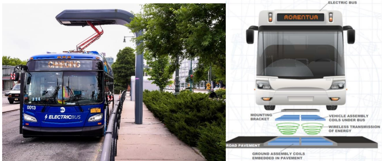
FIGURE 2-CONDUCTIVE (LEFT) AND INDUCTIVE (RIGHT) CHARGING. SOURCES: MTA AND MOMENTUM DYNAMICS
